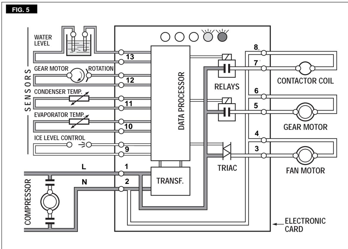
**NOTE.** The **ICE LEVEL CONTROL (INFRARED SYSTEM)** is independent of the temperature however, the reliability of its detection **can be affected by external light radiations** or by any sort of dirt and scale sediment which may deposit directly on the light source and on the receiver.
