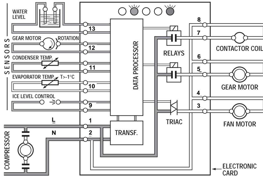
**NOTE.** If, after ten minutes from the compressor start-up, the evaporating temperature has not dropped down to a value lower than  $-1^{\circ}\text{C}$  ( $30^{\circ}\text{F}$ ) the evaporating temperature sensor detects such an abnormal situation and stops consequently the unit operation (first the compressor and 3' later the gear reducer). In this circumstance, the **5th warning YELLOW LED** will blink.
