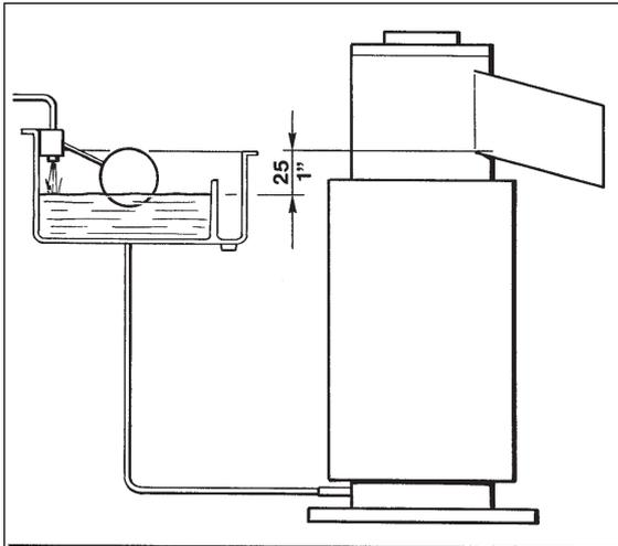
When the water level is above or below the correct one, adjustment can be performed by raising or lowering at the measure required, the water reservoir and its mounting bracket.
