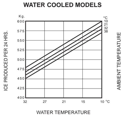
**NOTE.** The daily ice-making capacity is directly related to the condenser air inlet temperature, water temperature and age of the machine.
