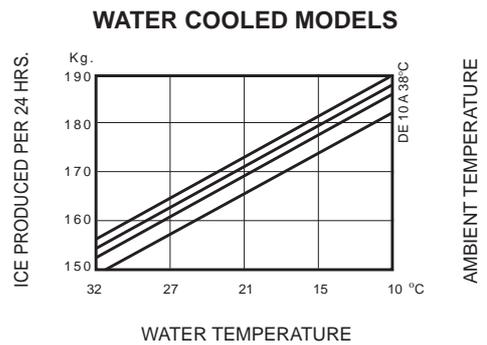
**NOTE.** The daily ice-making capacity is directly related to the condenser air inlet temperature, water temperature and age of the machine.
