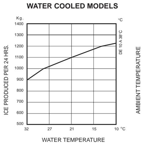
**NOTE.** The daily ice-making capacity is directly related to the condenser air inlet temperature, water temperature and age of the machine. To keep your **SCOTSMAN FLAKER** at peak performance levels, periodic maintenance checks must be carried out as indicated on maintenance section of this manual.
