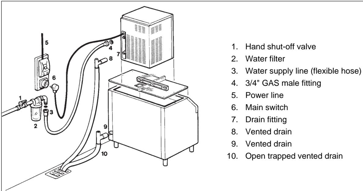
**WARNING.** This icemaker is not designed for outdoor installation and will not function in ambient temperatures below 10°C (50°F) or above 40°C (100°F). This icemaker will malfunction with water temperatures below 5°C (40°F) or above 35°C (90°F).
