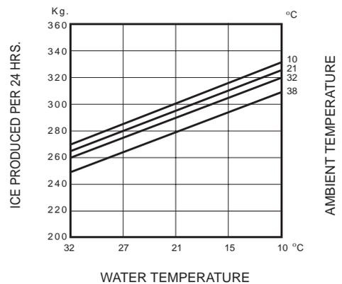
**NOTE.** The daily ice-making capacity is directly related to the condenser air inlet temperature, water temperature and age of the machine. To keep your **SCOTSMAN FLAKER** at peak performance levels, periodic maintenance checks must be carried out as indicated on maintenance section of this manual.
